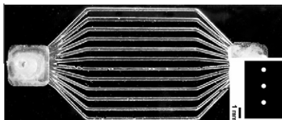
Fig. 2. Fin specimen used in the validation study consisting of twelve microchannels that fan from inlet and outlet network locations.
